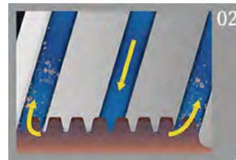
The waste and remaining solution are sucked to container through inlets
