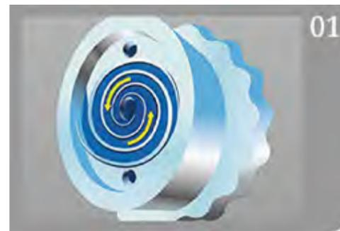
Solution is sprayed through the inlet of nozzle tip. It rotates clockwise.
